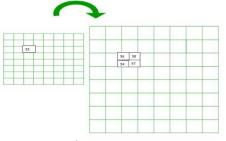
Fig 3: Showing how i<sup>th</sup> pixel of Low resolution image is interpolated onto high resolution grid
